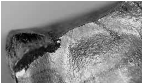
Excessive stress of the insert causes breakage.
